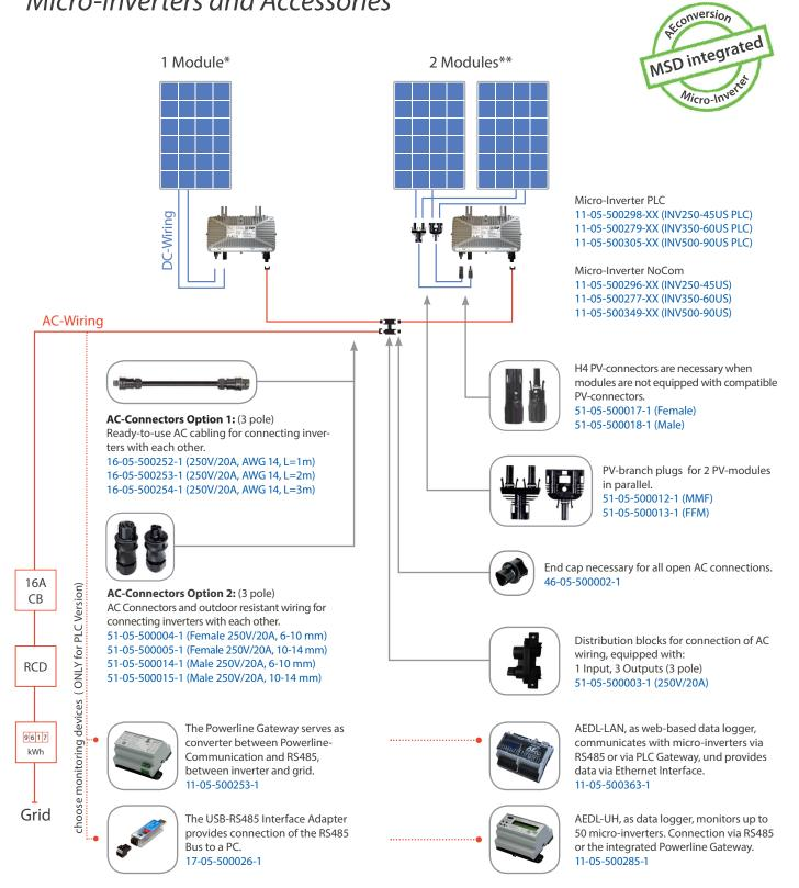
1 Module: 45V, 60V or 90V max. depending on inverter version
